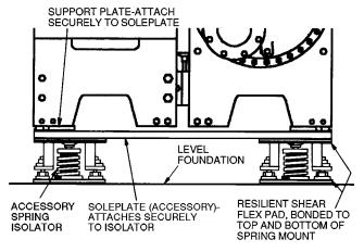
NOTE: The accessory spring isolators are supplied by Carrier for installation in the field.
